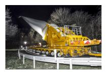
This means rotor blades can be swiveled over obstacles such as buildings and carriageway dividers...
