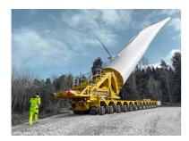
This rotor blade measures 84 meters long. The set-up angle of 60° provides the best possible maneuverability.
